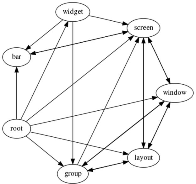
Each arrow can be read as "holds a reference to". So, we can see that a widget object holds a reference to objects of type bar, screen and group. Lets start with some simple examples of how the addressing works. Which particular objects we hold reference to depends on the context - for instance, widgets hold a reference to the screen that they appear on, and the bar they are attached to.
